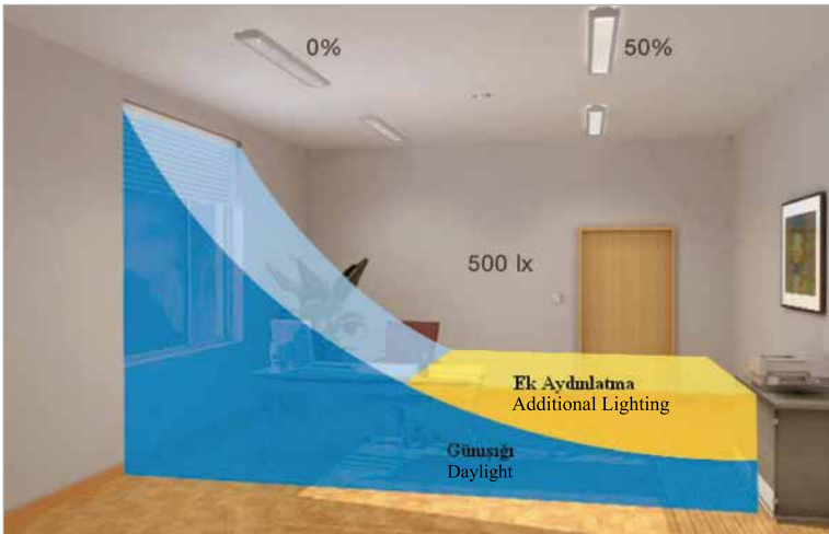
Dimming based on daylight dimming (Luxmate)
