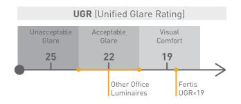
UGR (Unified Glare Rating) is the method used to calculate the glare caused by lighting fixtures. The UGR rating helps understand the extent of glare created by lighting fixtures. To maximize visual comfort, the Fertis offers a UGR<19 via a micro-prismatic diffuser.
