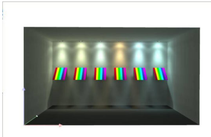
Fig. 205 All the spots are using the same colour filter, but have different light sources. From the left: Incandescent, Fluorescent 830, D65, high pressure sodium, metal halide ceramic and metal halide quartz
